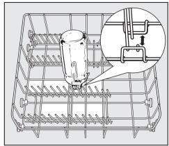
The bottle holder e.g. for milk or baby bottles, can be inserted into the bottom basket in more than one place. Position in any area marked white in the illustration. Do not place the insert in the corners of the lower basket, water cannot properly cover bottles in these areas.
